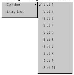
Use the SELECT ▲ or ▼ button to select the desired slot number from 1 to 10 of the ISS-6020 Swicher and press ENTER.
